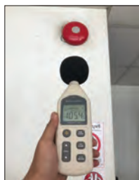
Photo 4.16 Check and Test Alarm Bell.
