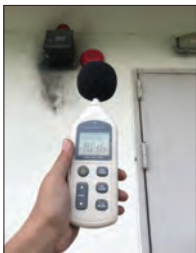
Photo 4.13 Check and Test Alarm Bell.
