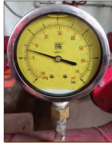
Photo 5.1.14 Pressure Suction 5 PSI.
