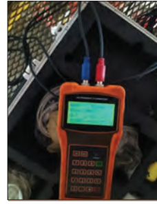
Photo 5.1.17 Flow 100% (Rated) 1003 GPM.
