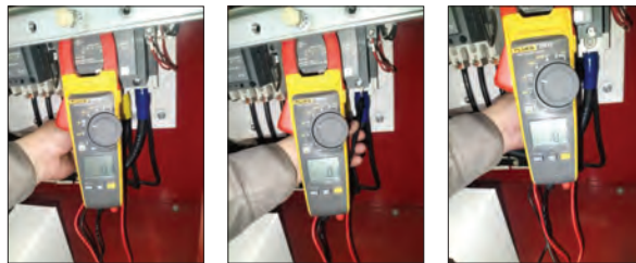
Photo 5.1.4 Check the resistance value of the fire pump electric motor winding.
