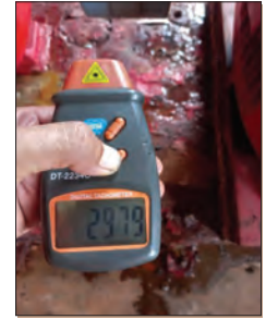
Photo 5.1.20 Speed 2979 RPM.
