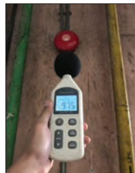
Photo 4.14 Check and Test Alarm Bell.
