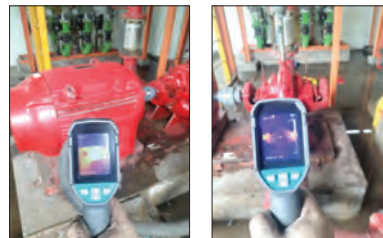
Photo 5.1.5 Check the electrical motor temperature.
