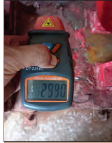
Photo 5.1.16 Speed 2990 RPM.
