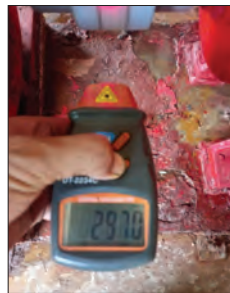
Photo 5.1.24 Speed 2970 RPM.
