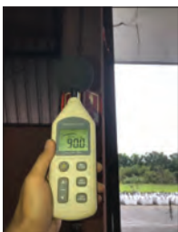
Photo 4.15 Check and Test Alarm Bell.
