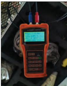
Photo 5.1.21 Flow 150% (Rated) 1502 GPM.
