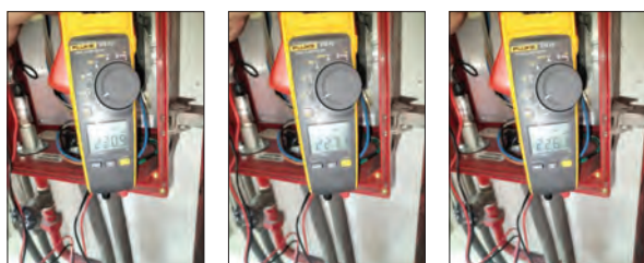
Photo 5.1.9 Check the voltage of the single phase jockey pump control cabinet.
